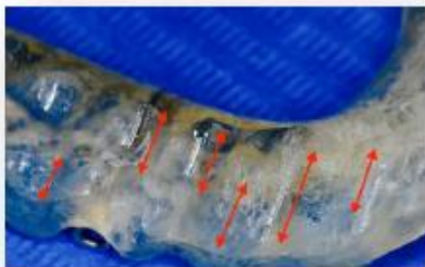
Example of grinding marks
