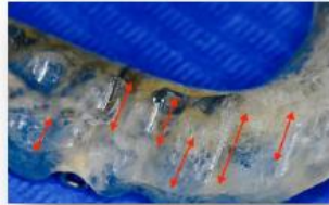
Example of grinding marks
