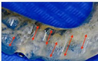
Example of grinding marks
