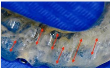
Example of grinding marks
