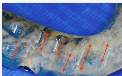
Example of grinding marks
